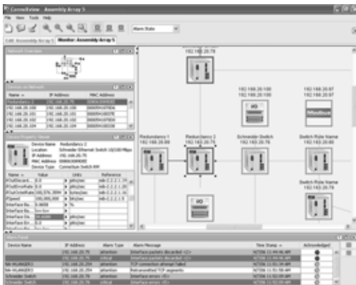
Automatic recognition of IP devices via the ConneXview diagnostic software for Ethernet industrial networks
