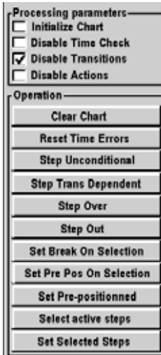
SFC control panel
