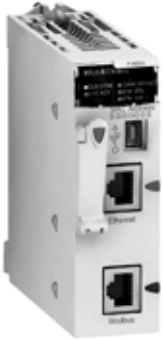
Ethernet port integrated in the BMX P34 2030/2040
